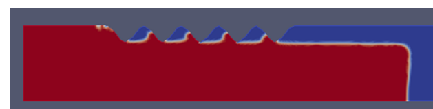
Figure 3. Results of nano simulation to replicate mould roughness.
